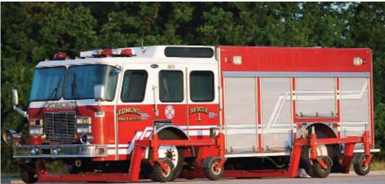
Raising or lowering the skid frame can increase or decrease the apparatus tires' degree of contact with the road, which in turn affects the amount of vehicle traction. If a driver commits a critical error, causing the vehicle to skid, the instructor can lower the vehicle and stop the skid.
